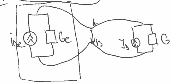
Millman Th refers to a star connection of n passive branches charact. by  $R_1, \dots, R_n$  and the electric potential of the terminals  $V_1 \rightarrow V_n$ .
