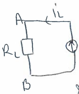
$$P = I_L^2 R_L = \frac{E^2 R_L}{(R_i + R_L)^2}$$
