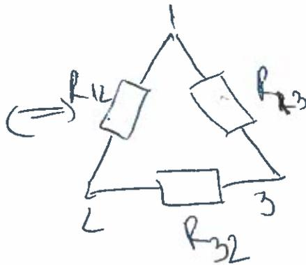
$$R_1 = \frac{R_{12} \cdot R_{13}}{R_{12} + R_{13} + R_{32}}$$
