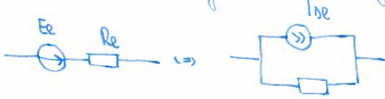
$$i_{be} + i_b = \underbrace{U_{AB} \cdot G_e}_{i_e} + \underbrace{U_{AB} \cdot G}_{i} = U_{AB} (G_e + G)$$
