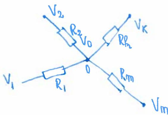
Refers to a star connection of "m" passive branches characterised by resistance  $R_1 \dots R_m$  and the terminal potential  $V_1, \dots, V_m$ . The common mode is mode 0. Under this circum., the potential of this mode is given by:
