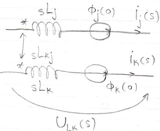
Every passive element is associated with an operational impedance and - for reactive elements - a generator equivalent with the initial conditions, and every active element is associated with an operational generator characterised by the Laplace transformation of the instantaneous characteristic of that generator.
