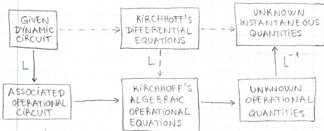
Laplace transformations are associated to the original circuit and to its instantaneous quantities, resulting in a corresponding operational circuit.
