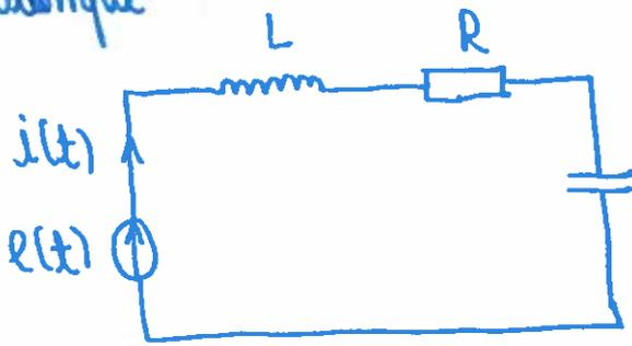
$$R = 24 \Omega \quad \omega L = \frac{1}{\omega C} = 5 \Omega$$
