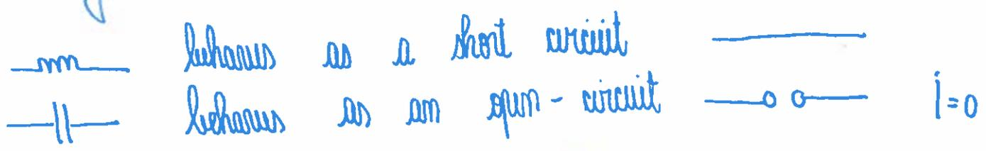
On the harmonics, where they don't have components, the voltage sources will be replaced by shortcircuits and the current sources will be replaced by open-circuit.
