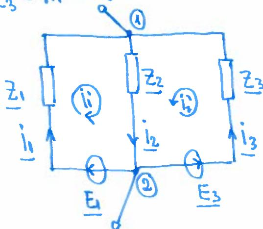
$$\underline{Z}_1 = R_1 + j(\omega L_1' + \frac{1}{\omega C_1}) \\ = 10 + j(30 - 10) = 10(1+2j)$$
