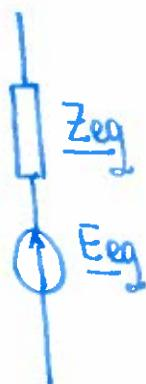
$$\underline{Z}_{eq} = \frac{1}{\frac{1}{\underline{Z}_1} + \frac{1}{\underline{Z}_2} + \frac{1}{\underline{Z}_3}} = \frac{1}{Y_1 + Y_2 + Y_3}$$
