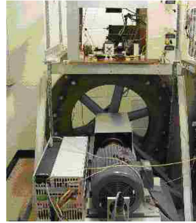
Fig. 21. Experimental setup showing guideway wheel.
