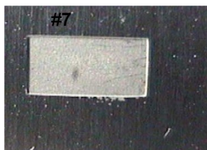
OD rubbing mark (length 16mm, width 8mm, depth 0.2mm);
