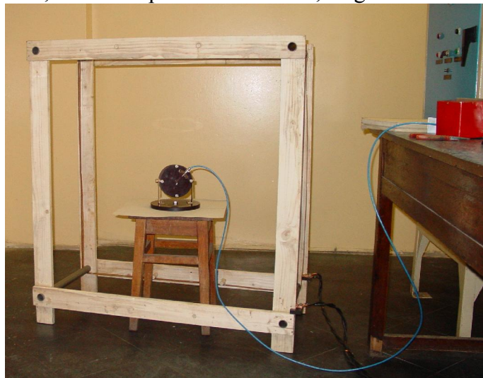
Fig. 8. The Helmholtz coil's picture with square section
