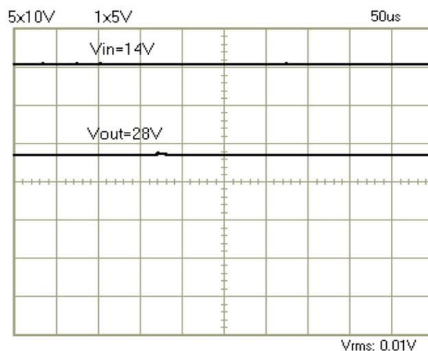
**Fig.9.** Input voltage  $V_{in}$  and output voltage  $V_{out}$  waveforms on oscilloscope PSC64i
