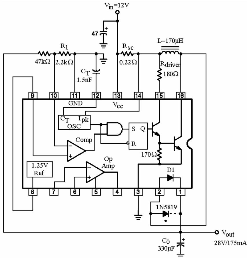
**Fig.6.** Switching power supply with  $\mu A78S40$  for dc-dc step-up converter
