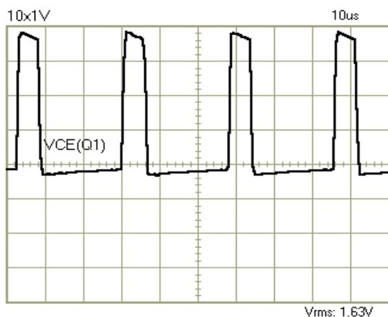
**Fig.10.** Voltage  $V_{CE}$  across switch  $Q1$  waveform
