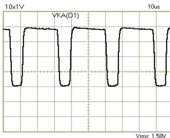
**Fig.11.** Voltage  $V_{KA}$  across diode  $D1$  waveform
