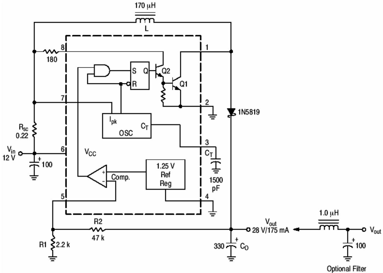
Fig.5. Switching power supply with MC34063 for dc-dc step-up converter
