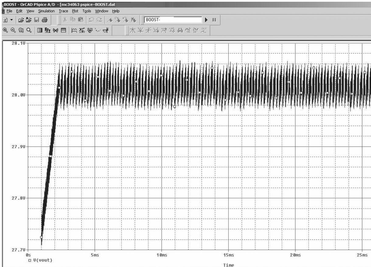
**Fig.8.** PSpice simulation waveform of the output voltage  $V_{out}$  on oscilloscope PSC64i
