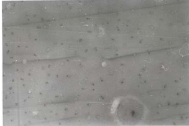
Fig. 3. Magnetic structures on stress free sheet.
