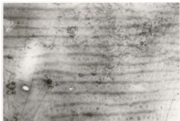
Fig. 8. Magnetic domains between two lines of irradiation.
