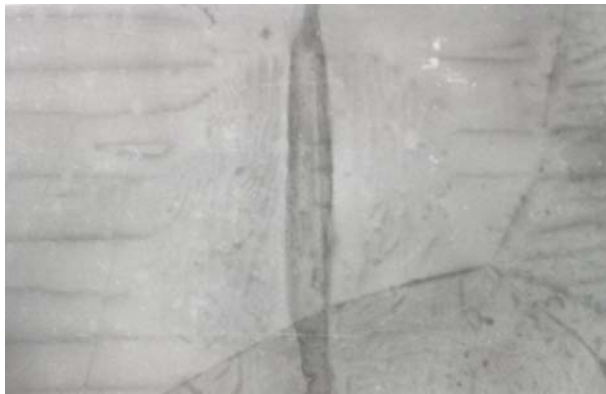
Fig. 4. Magnetic domains in stress sheet.
