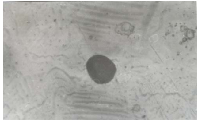
Fig. 5. Magnetic structures of a point stress.
