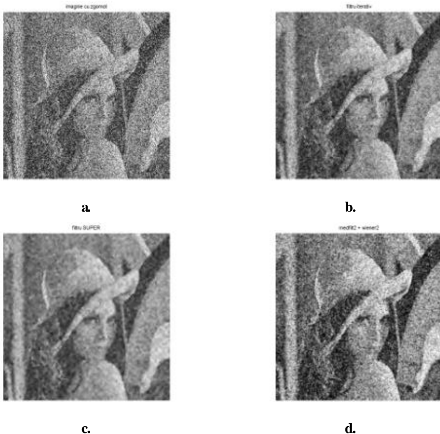
Fig 6. Images obtained by using the proposed filter an by cascading medfilt2 and wiener2 filters
