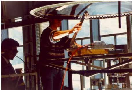
Figure 3: Splat –cooling device
